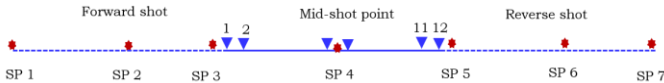
Figure. 3.7. A typical seismic refraction data acquisition layout and location of shot points for seismic refraction survey profile.
