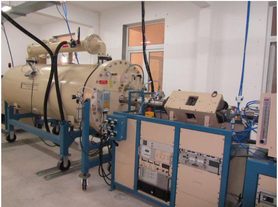
Figure 2.6. The HUS-5SDH-2 tandem pelletron accelerator system at the VNU University of Science in Vietnam
